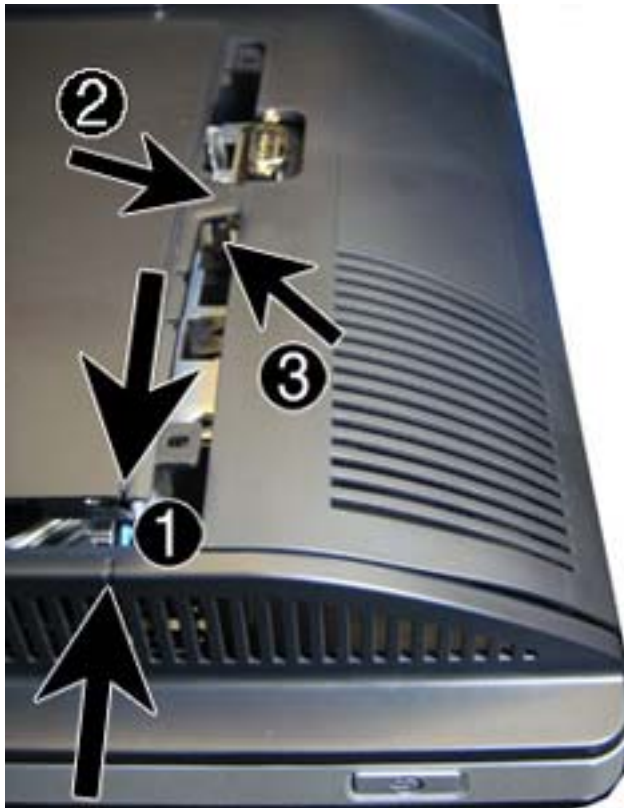
Figure 6-13 Access Panel Replacement
